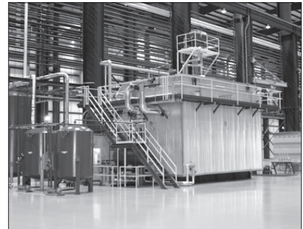
Figure 11: Micafil vapor phase system
